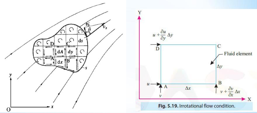
Circulation around regular curves can be obtained by integration. Let us consider the circulation around an elementary box (fluid element ABCD) shown in Fig. 5.19.
