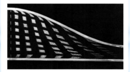
Deformation and rotation of fluid particles running through a narrowing channel
