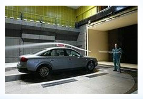
Example of a streakline used to visualize the flow around a car inside a wind tunnel.
