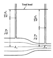
Fig. 5.6 Exchange between pressure head and velocity head
