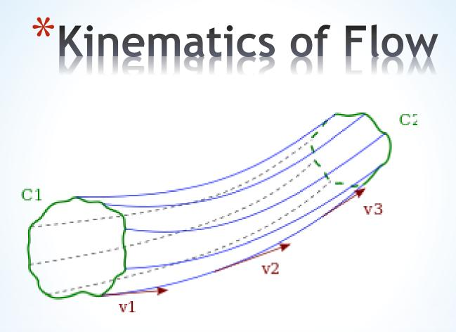
Solid blue lines and broken grey lines represent the streamlines. The red arrows show the direction and magnitude of the flow velocity. These arrows are tangential to the streamline. The group of streamlines enclose the green curves to form a stream surface.
