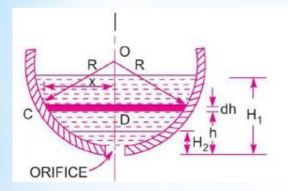
$$= \frac{\pi}{C_d \times a \times \sqrt{2g}} \left[ \frac{4}{3} R \left( H_1^{3/2} - H_2^{3/2} \right) - \frac{2}{5} \left( H_1^{5/2} - H_2^{5/2} \right) \right] \quad \dots (7.13)$$
