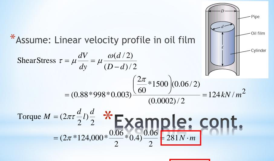
Power  $P = M\omega = 281*157.1 = 44,100 N \cdot m/s = 44.1 kW$
