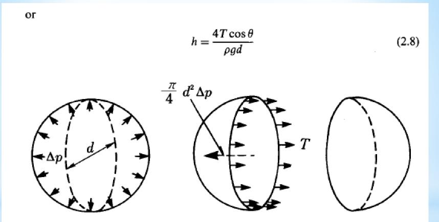
Fig. 2.6 Balance between the pressure increase within a liquid drop and the surface tension
