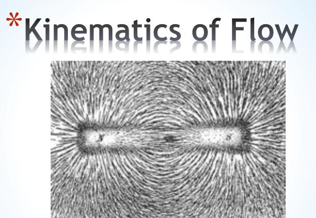
The direction of magnetic field lines are streamlines represented by the alignment of iron filings sprinkled on paper placed above a bar magnet
