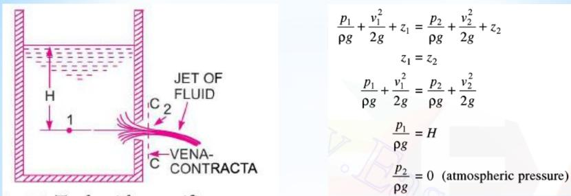
ig. 7.1 Tank with an orifice.
