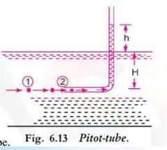
$\frac{p_1}{\rho g} + \frac{v_1^2}{2g} + z_1 = \frac{p_2}{\rho g} + \frac{v_2^2}{2g} + z_2$ But  $z_1 = z_2$  as points (1) and (2) are on the same line and  $v_2 = 0$ .  $\frac{p_1}{\rho g} = \text{pressure head at (1)} = H$
