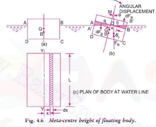
$$\therefore \quad \text{Meta-centric height} \qquad = GM = \frac{I}{\forall} - BG.$$
