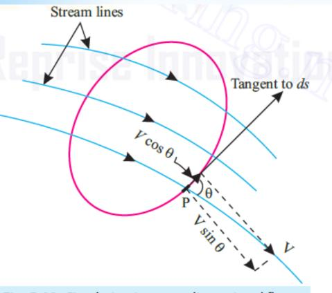
Fig. 5.18. Circulation in a two-dimensional flow.
