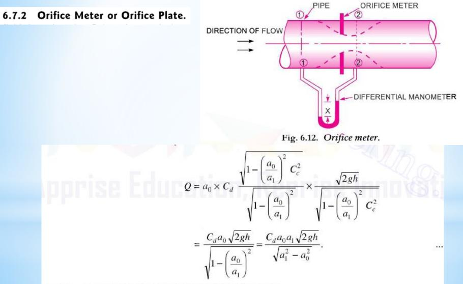
where  $C_d =$ Co-efficient of discharge for orifice meter.
